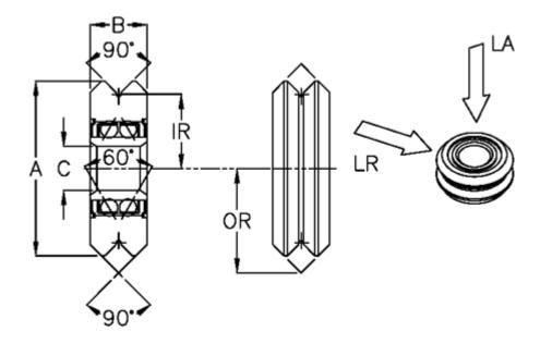
$\begin{array}{ll} \mbox{Diameter A} & = 19.58 \\ \mbox{Hole size C} & = 4.76 \\ \mbox{Internal radius IR} = 7.95 \\ \mbox{Outer radius OR} & = 11.89 \\ \mbox{Width B} & = 7.87 \end{array}$
